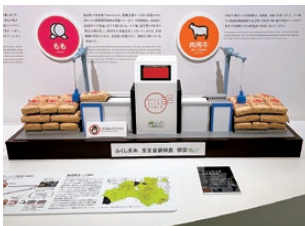
Model of a machine used to screen radiation of rice in all bags
