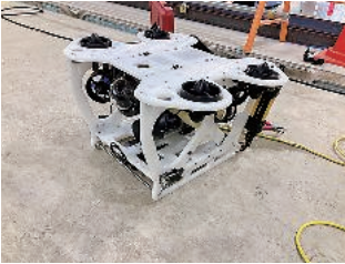
"Ryuzu" ROV with a Doppler Velocity Log
