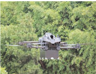
"Aegis One," a hydrogen fuel cell-powered logistics drone
