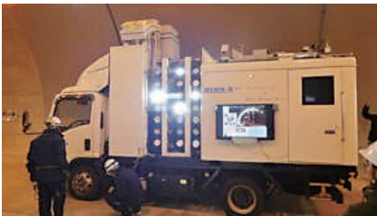
A mobile high-speed 3D tunnel inspection system (MIMM-R)
